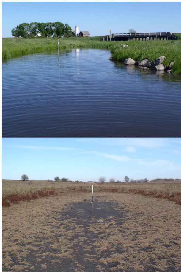
FIGURE 2 Oxbows, with water (top) and dried up (bottom), in the North Raccoon River Basin of West Central Iowa, USA. The data loggers that recorded stage height, mounted on steel fence posts, are visible
